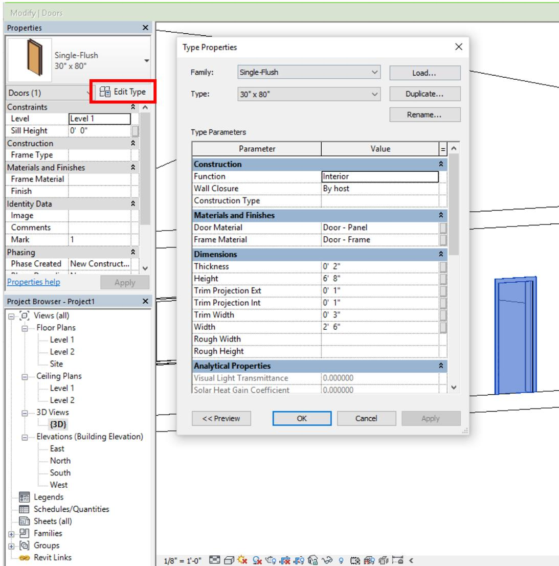
If you would like a completely different door (this procedure also applies to windows, walls, columns, etc.), click “door” under the architecture tab as if you were going to add a new door to the project. Under the “Modify” tab on the toolbar is a command called “Load Family”. Click it, and this window should appear:
