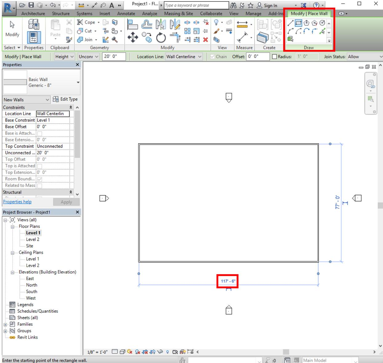
If you made a mistake in your initial drawing, you can always double click on the dimension in blue, and change it manually by typing in the correct value. Once you are done modifying the wall, click the “esc” button.
