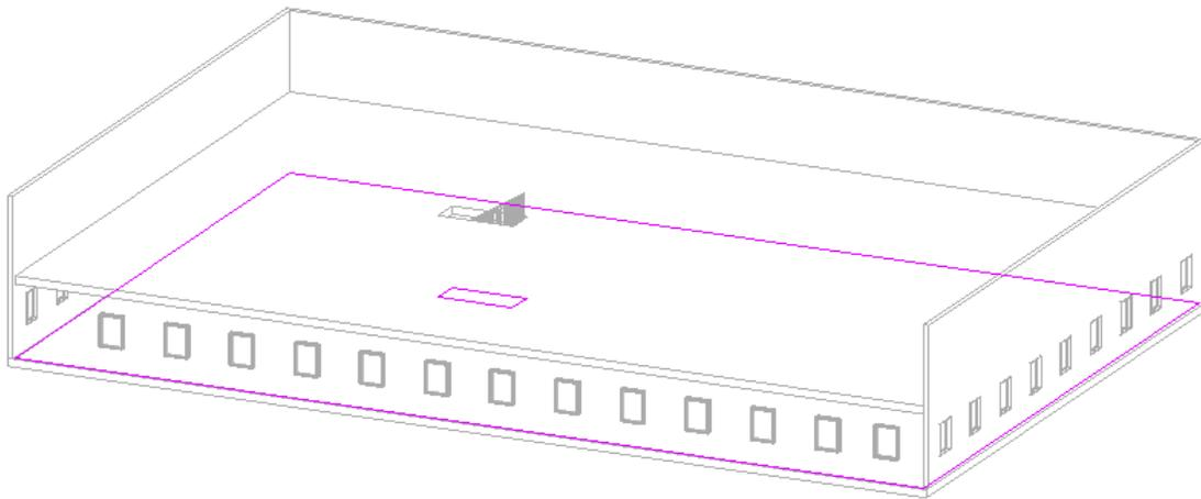
Using the compass in the top right of your screen, click on “TOP” to get a overhead view of your stairs. In the “Modify | Edit Boundary” tab of the toolbar, click the rectangle icon and draw a rectangle around your stairs, so that you make a “cut” or “gap” in your floor.
