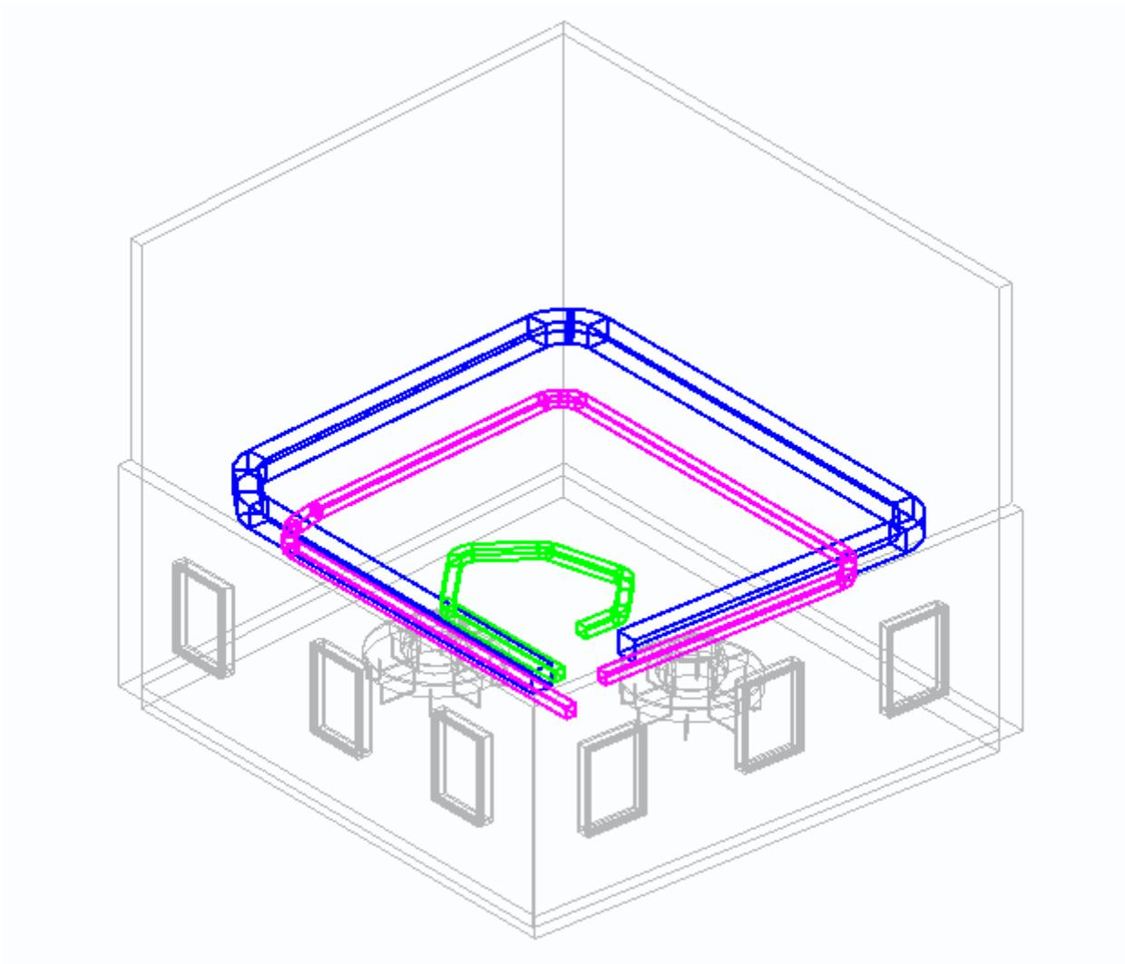
**NOTE:** Be careful of the offset setting. Use the 3D view to make sure you aren't clashing with architectural components such as ceilings, floors, lights, other ducts, etc.
