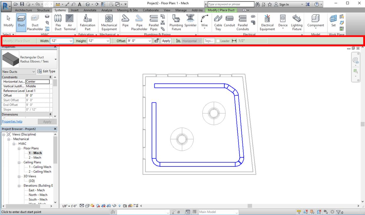
You can change the duct type (Exhaust, Return, or Supply air) by clicking on its “System Type” in the properties tab. Each type has a different color. See the example below:
