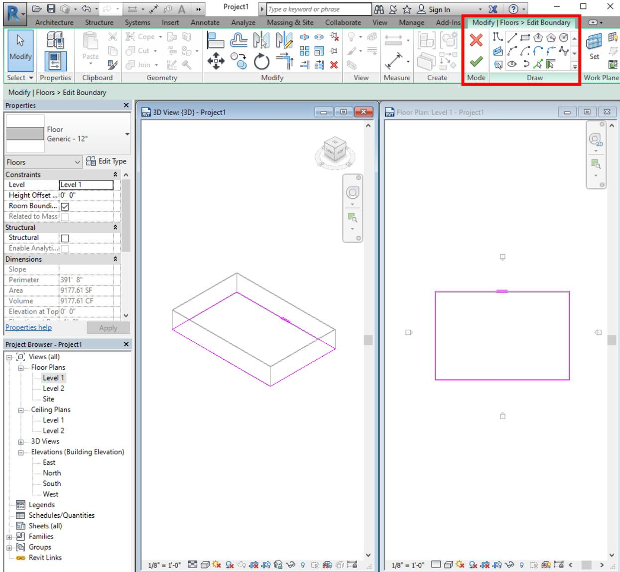
The procedure for ceilings is almost the exact same. After clicking “ceiling” under the “architecture” tab, it will prompt you to create an automatic ceiling or if you want to sketch the ceiling manually. If you have a simple wall design (such as a single rectangle), you can use an automatic ceiling. If you have a more complex wall design shape, click sketch ceiling. The procedure to sketch your ceiling boundary is the same as the floor boundary.
