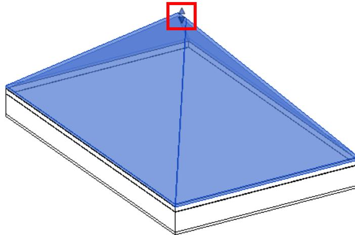
If you would like to change the height of the roof, click and drag the arrows at the peak of the roof.
