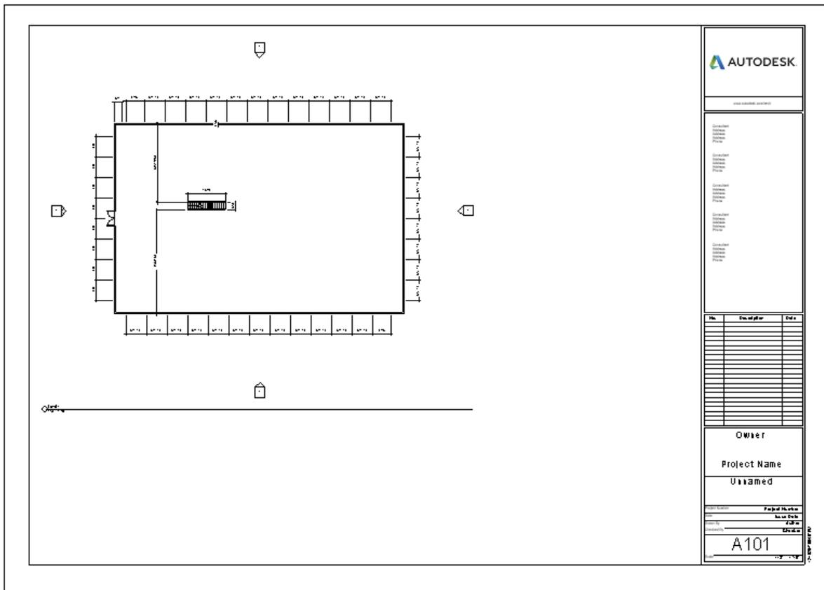
To change the size of the plan on your sheet, go to the plan you are trying to put on your sheet, and change the size ratio of the drawing. You can do this by going to the bottom toolbar (see part 3: Views of this tutorial for help) and clicking the ratio. The default is set to  $1/8'' = 1'-0''$ . To make the view smaller on your drawing, make your ratio smaller (i.e.  $1/6'' = 1'-0''$ ). The size will decrease significantly.
