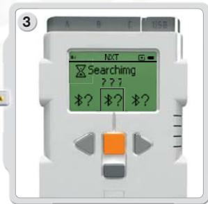
3 Depending on how many are detected in the area, the Bluetooth devices will appear in a list on the NXT display after a few seconds.
