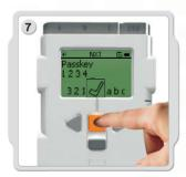
If you connect to a device for the first time, your NXT asks for a Passkey. Just press Enter to use the default passkey 1234 or make up your own code. The other Bluetooth device must know your passkey in order to confirm the connection. This means the two NXT bricks need to enter the same passkey in order to connect.
