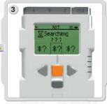
Depending on how many are detected in the area, the Bluetooth devices will appear in a list on the NXT display after a few seconds.
